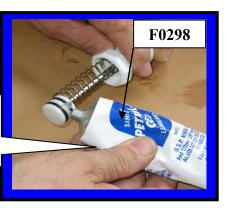
Installing **Plunger Assembly** into Faucet body
