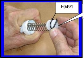
Install **O-rings** onto plunger
