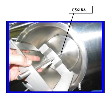
Re-install the large **faceplate** on the machine. First place the faceplate **bushing** onto the beater shaft. Then slide face plate onto the four studs. Install the faceplate knobs and tighten evenly until the faceplate O-ring is snug against the cylinder.
