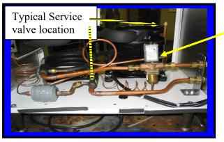
Valves automatically open on pressure increase, close on pressure decrease. <u>Adjustment:</u> To raise valve opening point, turn adjusting screw, on top of valve, counterclockwise. To lower operating point, turn clockwise. Opening point of valve should be raised just enough to cause valve to close during compressor stand-by periods.
