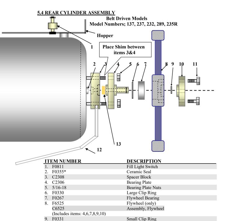
\*Note: F0355 is the part # for the Spring Seal Assembly which includes the ceramic seal. (No. 2 above)
