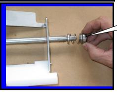
Step 5: Install spring seal F0355
