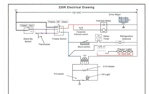
NOTE: When refrigeration solenoid closes, condenser pressure drops. At 10 psi the condensing unit shuts off. When the refrigeration solenoid opens, condenser pressure rises, At 35 psi the condensing unit will cycle on after an approximate 2 minute delay.
