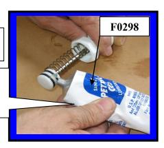
Installing **Plunger Assembly** into Faucet body
