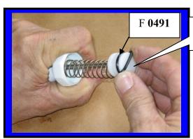
Install **O-rings** onto plunger
