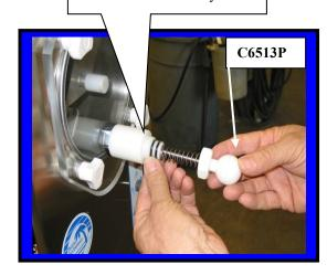
Installing **Faceplate** onto front of Machine.
