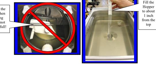
When the cylinder is full and the hopper is filled to one inch from the top, the machine is ready to run. Turn on by selecting the "right" (snowflake) position of **<u>both</u>** switches on the front panel.
