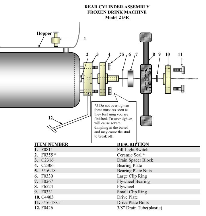
\*Note: F0355 is the part number for the <u>Spring Seal Assembly</u> Which includes the ceramic seal (No.2 above)
