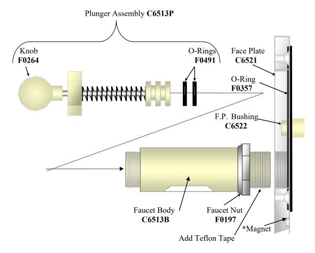
\*Motor Disconnect Magnet (Motor will not operate when faceplate is removed)
