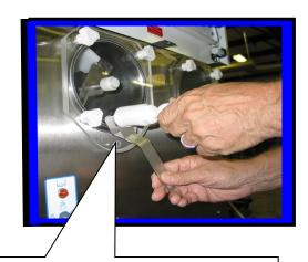
Align Faucet Assembly opening to bottom of faceplate then tighten nut
