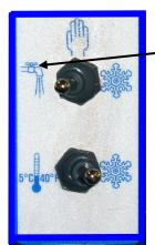
**Cleaning Operation -** The drive motor will run in the **faucet** position to allow a stirring action of the rinse water while cleaning.
