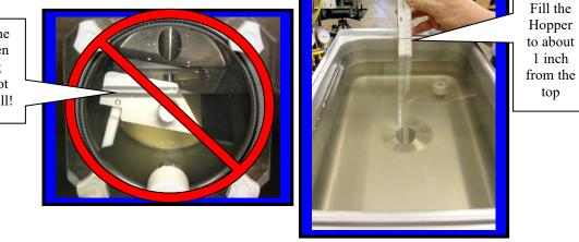
When the cylinder is full and the hopper is filled to one inch from the top, the machine is ready to run. Turn on by selecting the "right" (snowflake) position of **<u>both</u>** switches on the front panel.
