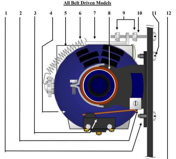
1. U-Nuts (2) 5/16-18 2. Microswitch Friction Plate F tba 3. Microswitch F0346 4. Motor (ONLY) F732 5. Motor Assembly C732 (Includes items: 1,2,3,4,6,9.13. 6. Motor Stop Bracket F1203 7. Tension Spring Lg F0469 8. Spring Adjustment Bracket F4202A 9. Motor Bearing F0738 10. Lock nuts (2) <sup>1</sup>/<sub>4</sub>-20 11. TCC Adjustment Screw <sup>1</sup>/<sub>2</sub>-20x3" 12. Screw, Mtr mt. 5/16"x 18 phs 13. Motor Pulley F0471
