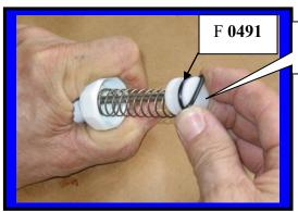
Install **O-rings** onto plunger
