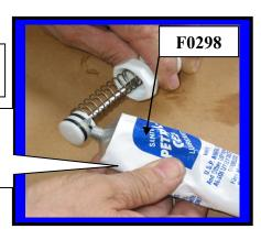
Installing **Plunger Assembly** into Faucet body
