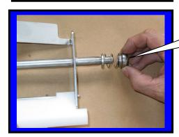
Step 5: Install spring seal F0355
