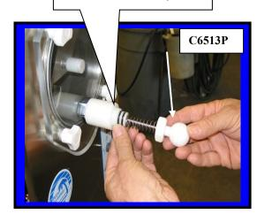
Installing large **Faceplate** onto front of Machine.
