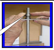
Step 7: Install beater bar C6519 into cylinder.
