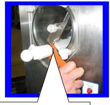
Align Faucet Assembly opening to bottom of faceplate then tighten nut
