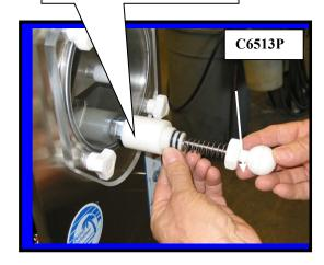
Installing **Faceplate** onto front of Machine.
