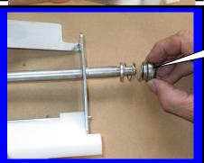
Step 5: Install spring seal F0355
