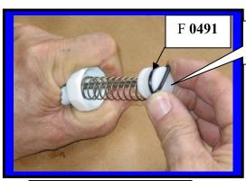
Install **O-rings** onto plunger
